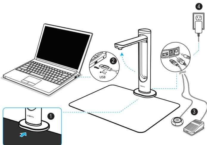
NOTE: Ensure the scanning pad is in contact with the scanner base.
